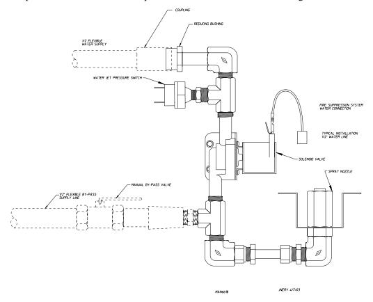
**WARNING:** If the water in the supply line or water solenoid valve freezes, the S.A.F.E. system <u>will</u> **be** INOPERATIVE!!
