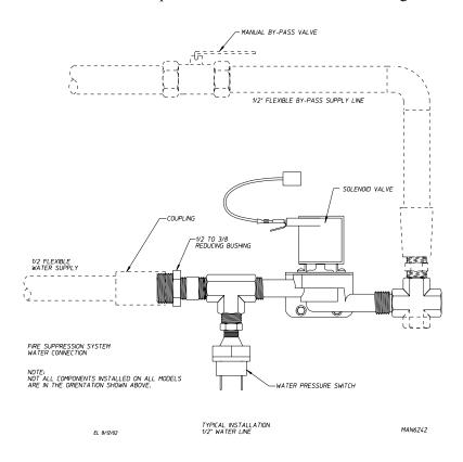
**WARNING:** If the water in the supply line or water solenoid valve freezes, the S.A.F.E. system <u>will</u> **be** INOPERATIVE!!
